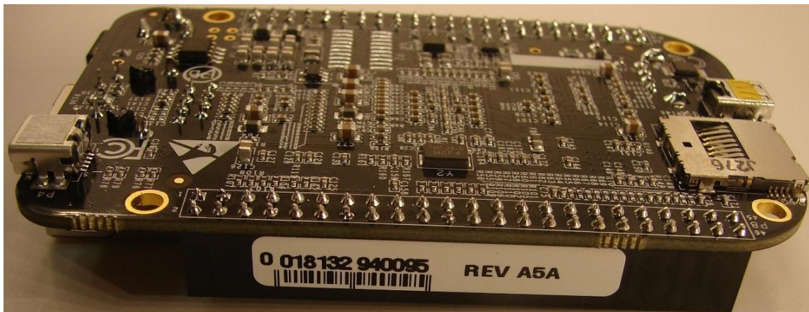
Fig. 5.81: Third Phase Serial Number and Revision Location
