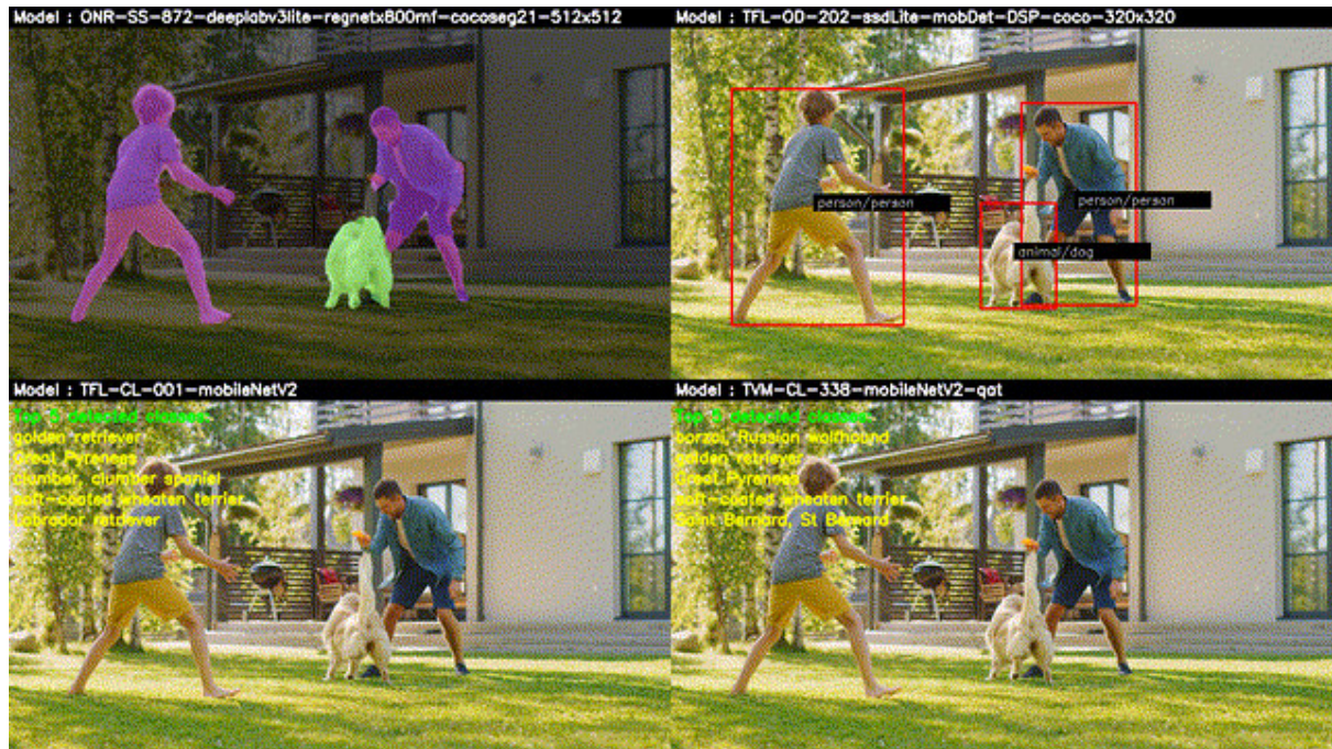
Fig. 3.36: Sample output showing single input, mutli-inference output
