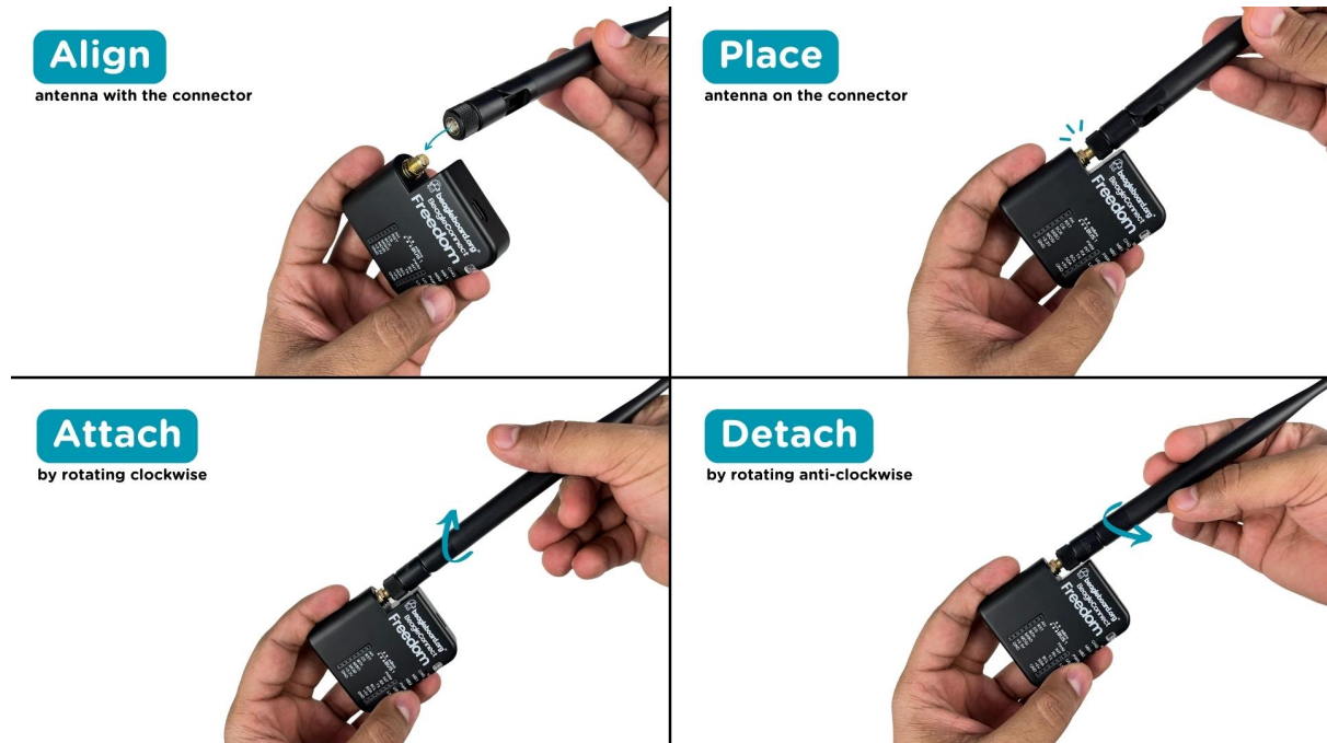
Fig. 12.1: Attaching antenna to BeagleConnect Freedom
