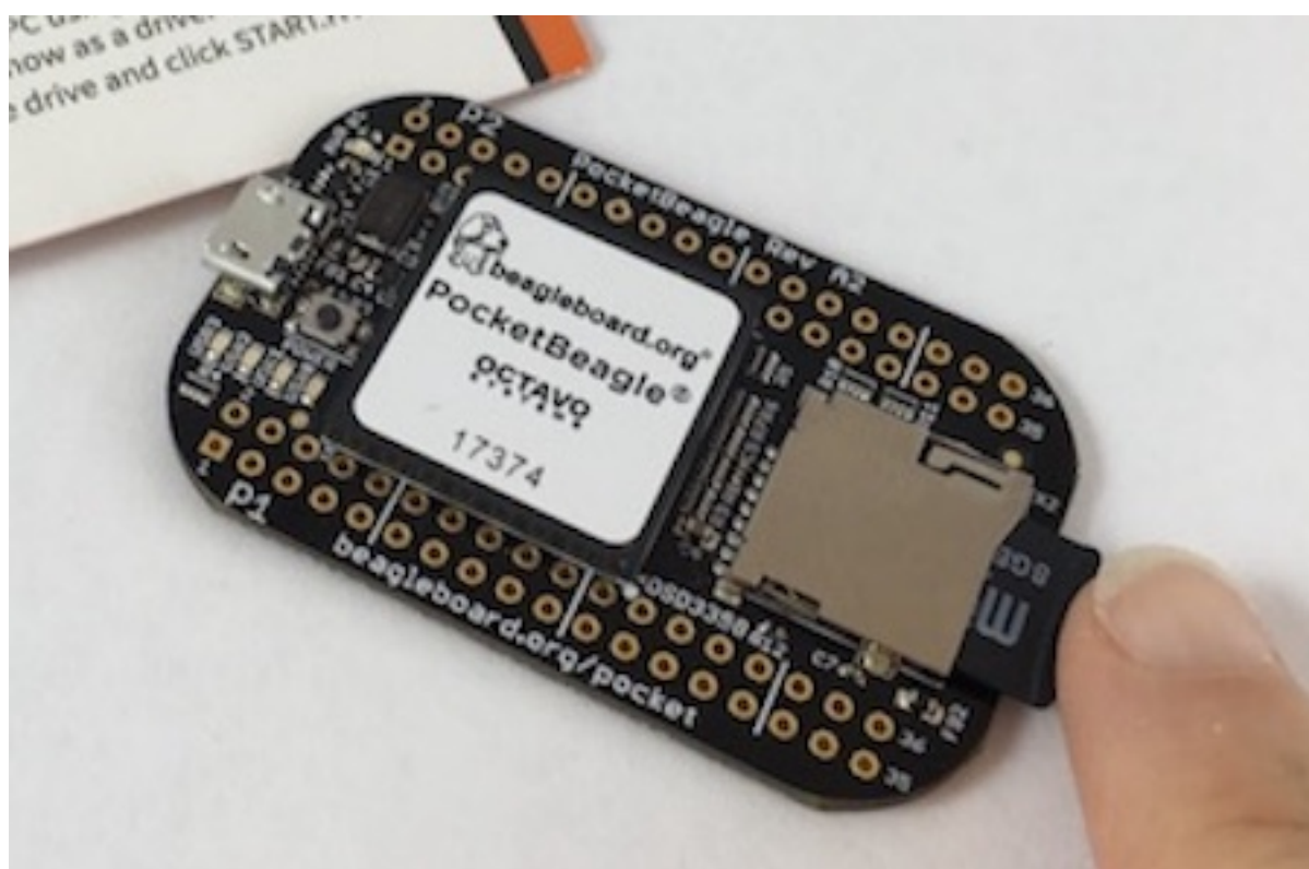
Fig. 11.11: Insert the microSD Card into PocketBeagle
