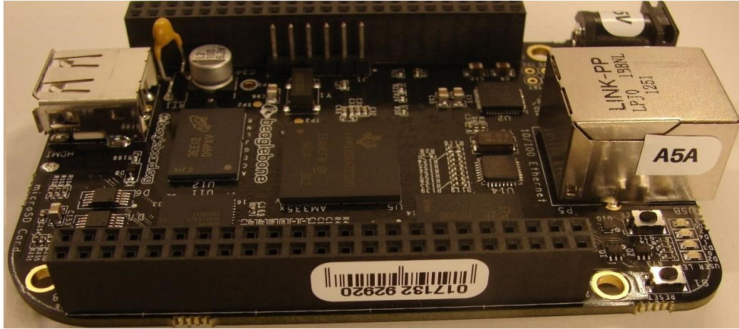
Fig. 5.80: Second Phase Serial Number and Revision Location
