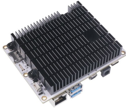
Fig. 3.63: BeagleBone AI-64 back with heatsink at 45° angle
