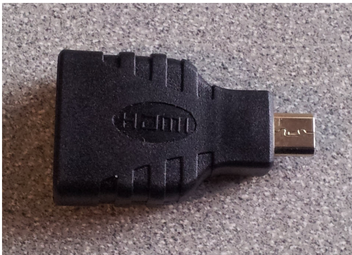
Fig. 15.39: Female HDMI-to-male microHDMI adapter
